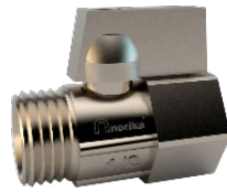
SKU: MBVCRN DZR BRASS MINI BALL VALVE MxF [NICKEL PLATED] Size availability: 1/4" to 1"
