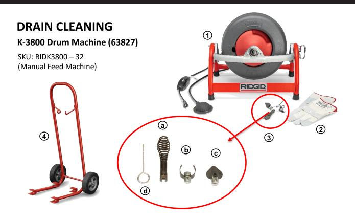
The K-3800 Drum Machine is a powerful, easy to transport, versatile machine for cleaning indoor drains. For 3/4" (20 mm) to 4" (110 mm) Drain Lines. Rugged, corrosion-resistant molded cable drum won't dent or rust. The drum tilt adjusts for proper cable feed angle. Inner-drum guards against cable flip-over inside the drum. Powerful 1/10 HP universal motor spins cable at 240 RPM. When cable hits blockage, motor gears down automatically to deliver more power and enhance operator control.
