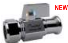
SKU: MBVCRPFN015 \frac{1}{2} " DZR BRASS [PFxCC] MINI BALL VALVE [CHROME PLATED]
