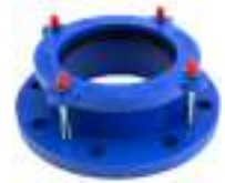
SKU: DIFA-EPC HEAVY DUTY DUCTILE IRON FLANGE ADAPTOR C/W EPOXY COATED Size availability: 3" to 12"
