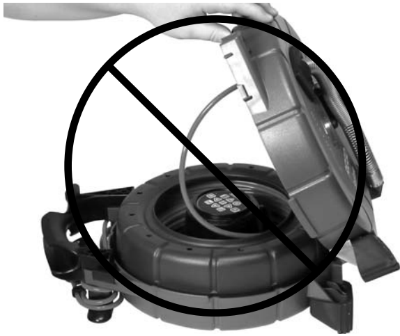
Figure 10 – Do Not Allow Cable to Uncoil Freely
