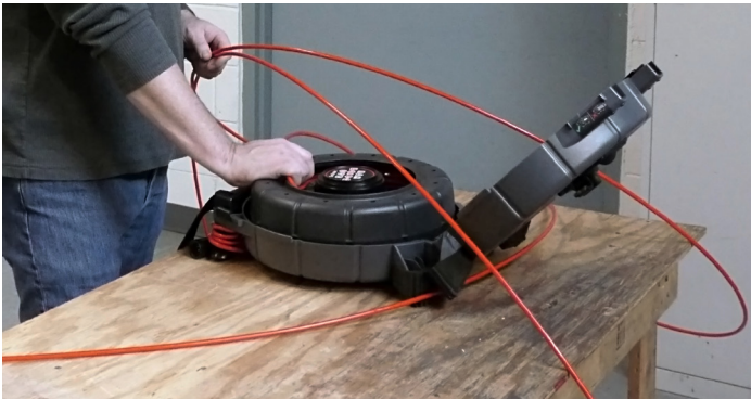
Figure 1 – Drum properly seated in casing
