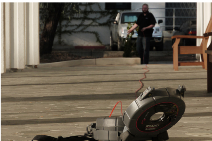
Figure 2 – Straightening the push cable
