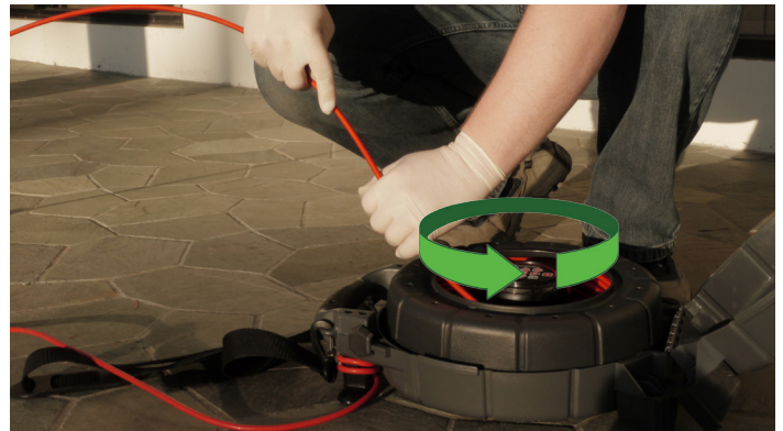
Figure 3 – Rotate drum to properly wind the push cable
