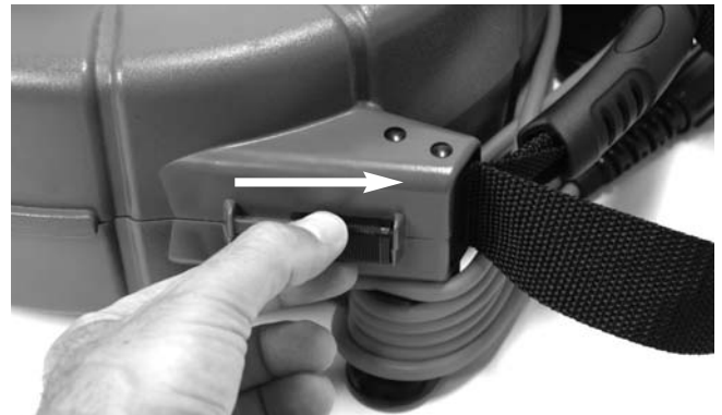
Figure 4 – Unlatching the microReel Case
