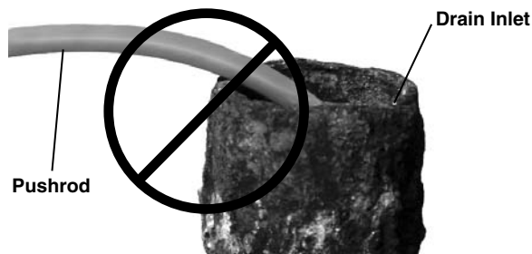
Figure 23 – Avoid Pulling At Sharp Angles
