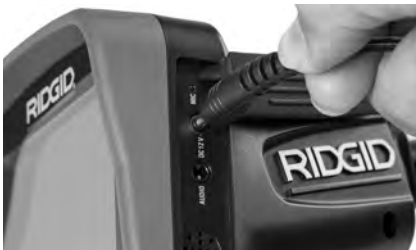
Figure 6 – Powering the Unit with AC Adapter
