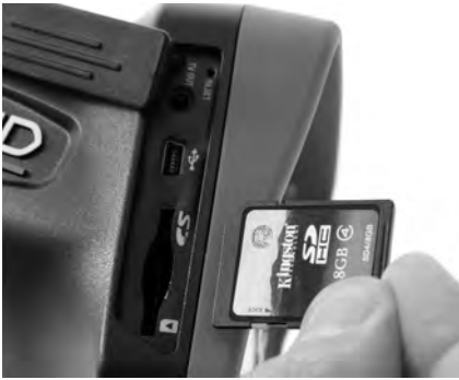
Figure 9 – Inserting the SD Card
