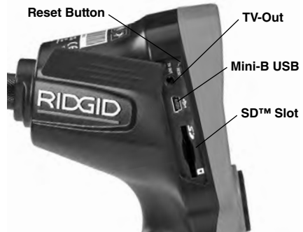
Figure 4 – Left Side Port Cover
