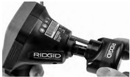
Figure 18 – Camera Connector Plug Installed
