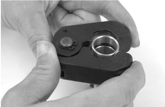
Figure 11 – Installing Press Ring onto Fitting (Need Pictures)
