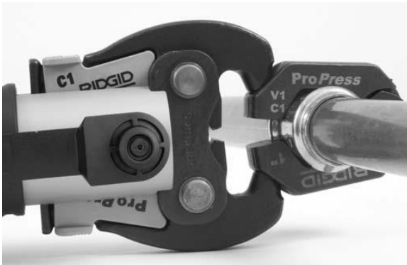
Figure 12 – Attaching Actuator to Press Ring (Need Pictures)
