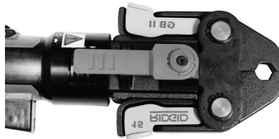
Figure 3 – Fully Closed/Locked Mounting Pin
