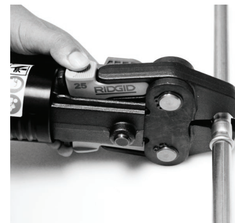
Figure 5 – Opening The Scissor-Style Jaws
