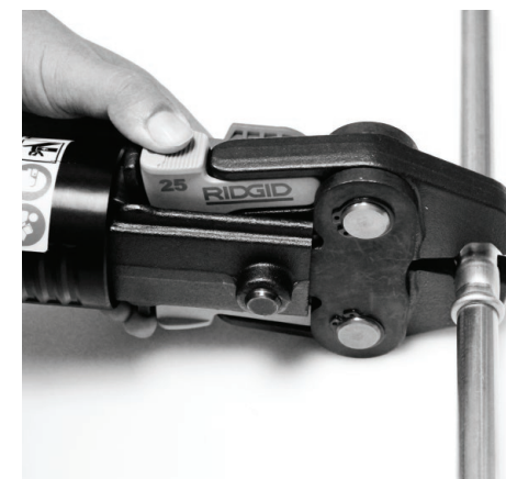
Figure 5 – Opening The Scissor-Style Jaws
