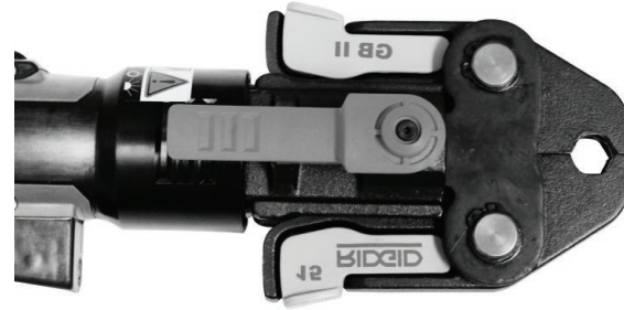
Figure 3 – Fully Closed/Locked Mounting Pin
