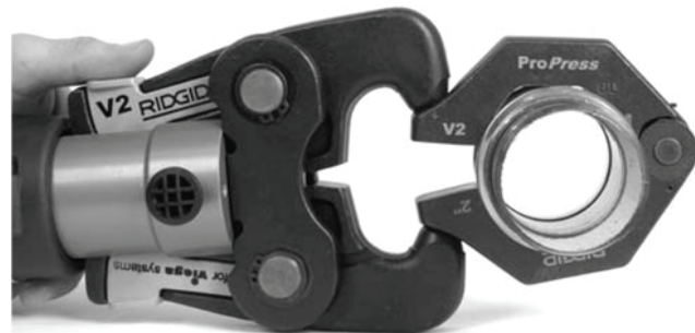
Figure 9 – Attaching Actuator To Press Ring
