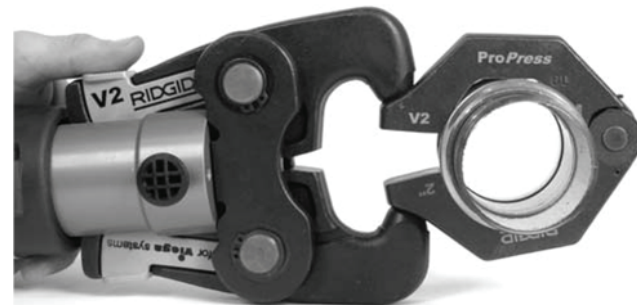
Figure 9 – Attaching Actuator To Press Ring
