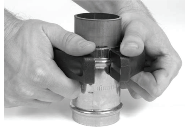
Figure 8 – Installing Press Ring Onto Fitting
