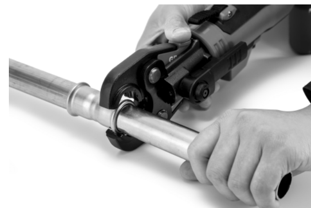
Figure 5 – Opening The Scissor-Style Jaws
