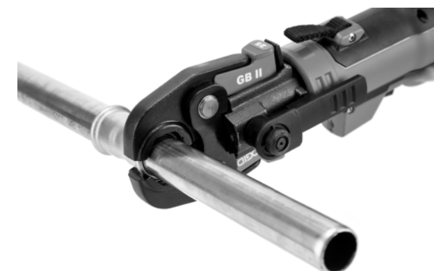
Figure 6 – Placing Scissor-Style Jaw Set Around Fitting
