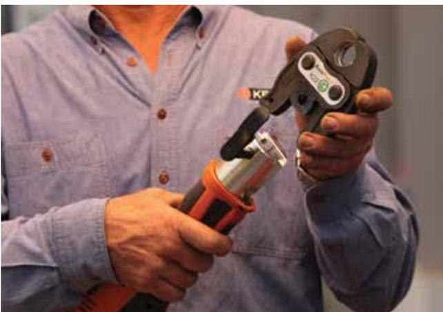
**5.** Select pressing jaw according to the fitting dimension and insert into the pressing machine. Arrest the locking bolts of the machine. Check the jaws are free from debris and in good working order.
