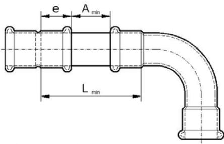
Minimum spacing between two press points. **See table 1.**
