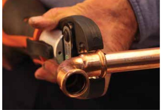
**7.** Check the fitting outer edge still lines up with the marking. Open the pressing jaw and close it around the fitting so the raised bump in the fitting rests inside the groove of the pressing jaw.
